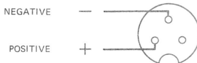
Fig. 2-3 Terminations on DC Supply Connector (viewed on wiring side).
